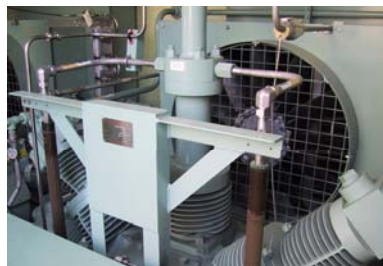
High pressure hydrogen compressor 110MPa, 200Nm 3 /h
