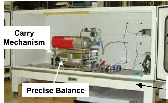
Precise balance for weight method F.S.:52kg, Minimum reading: 0.01g
