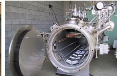
Temperature controllable air tight chamber Range: -40-85 deg.C
