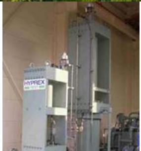
Hydraulic pressure 120MPa cycle, 300MPa burst
